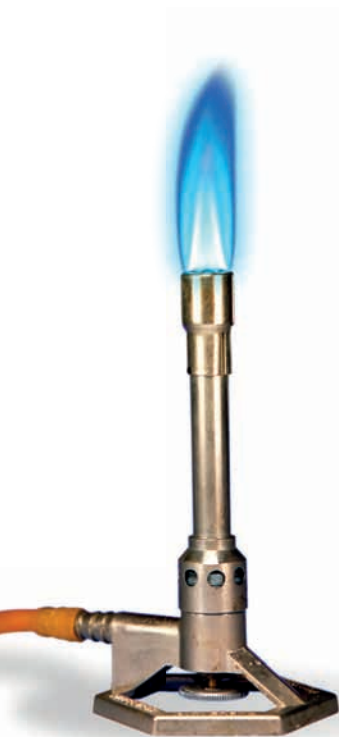
The Bunsen burner controls the combustion of methane, \text{CH}_4 , and is often used as a source of heat in the laboratory.
